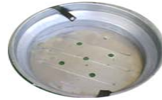
Top View Shows Gas Vents
